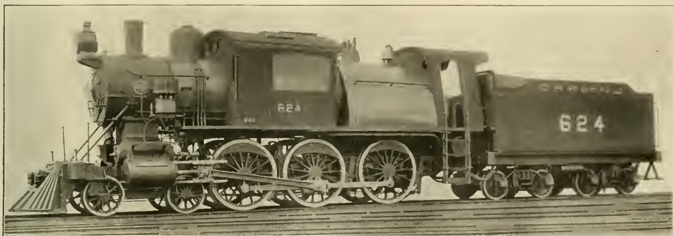
TEN-WHEEL PASSENGER LOCOMOTIVE—CENTRAL RAILROAD OF NEW JERSEY
